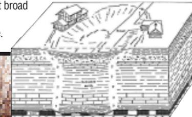
Subsidence is usually greatest at the center of the trough and it progressively decreases until the limit of the impacted surface area is reached. Horizontal ground movements also occur within a subsidence trough. Structures near the center of the trough
